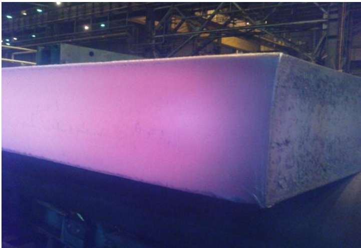
hot cutting of slab 250 mm thickness
